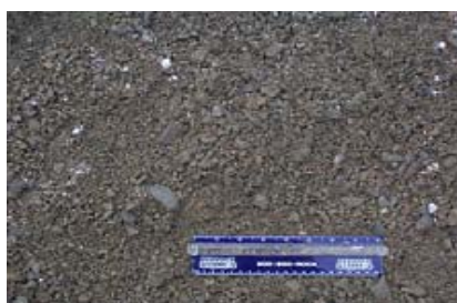
Figure 7. Surface layer of crushed stone
